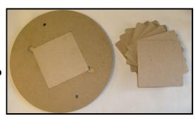
This pocket receives the  $5 \frac{1}{2}$  square inserts. The inserts are removed by lifting a corner of the insert. Two machined finger slots at opposite corners of the pocket allow for finger access.
